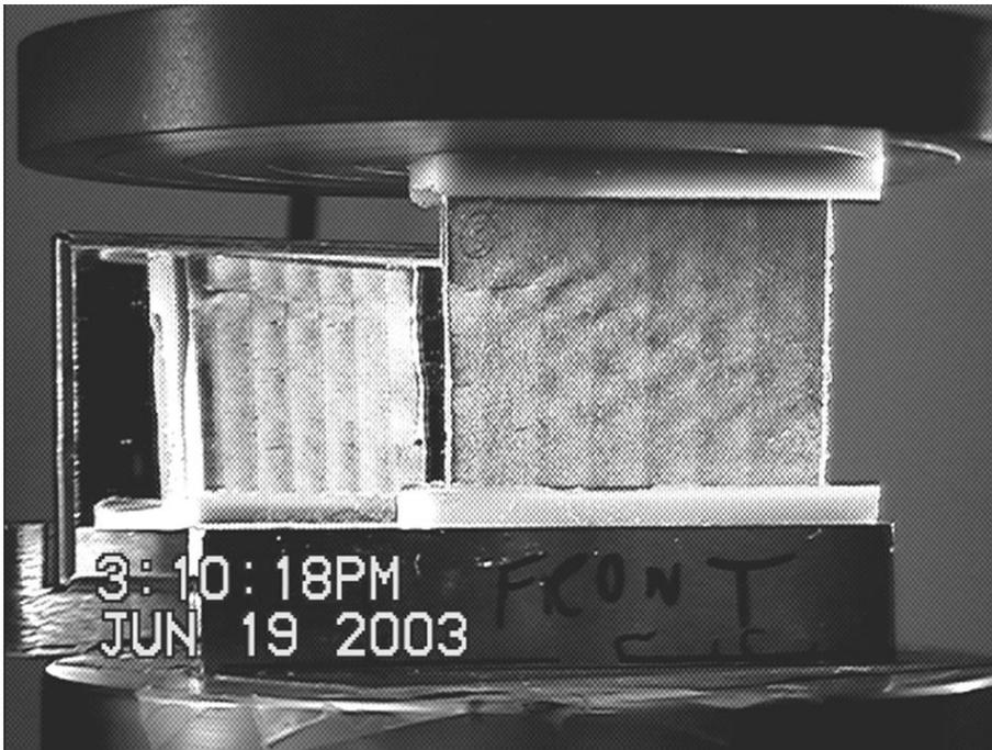
**Figure 1. Instantaneous snapshot of an AC multi-wall board undergoing an ECT test. The A-flute side (in the mirror view) has already failed while the C-flute side displays a buckling pattern.**
