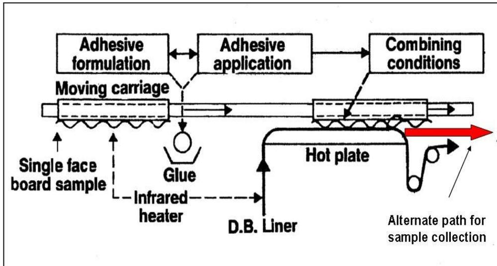
**Figure 3. Schematic of the IPST double backer simulator used to apply varying glue types at various levels to single face samples.**
