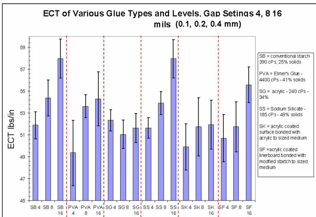
**Figure 4. ECT of test boards made on the double backer simulator with varying adhesive type and adhesive levels. Numeric suffix denotes the adhesive applicator doctor gap setting in units of 0.001" (mils).**
