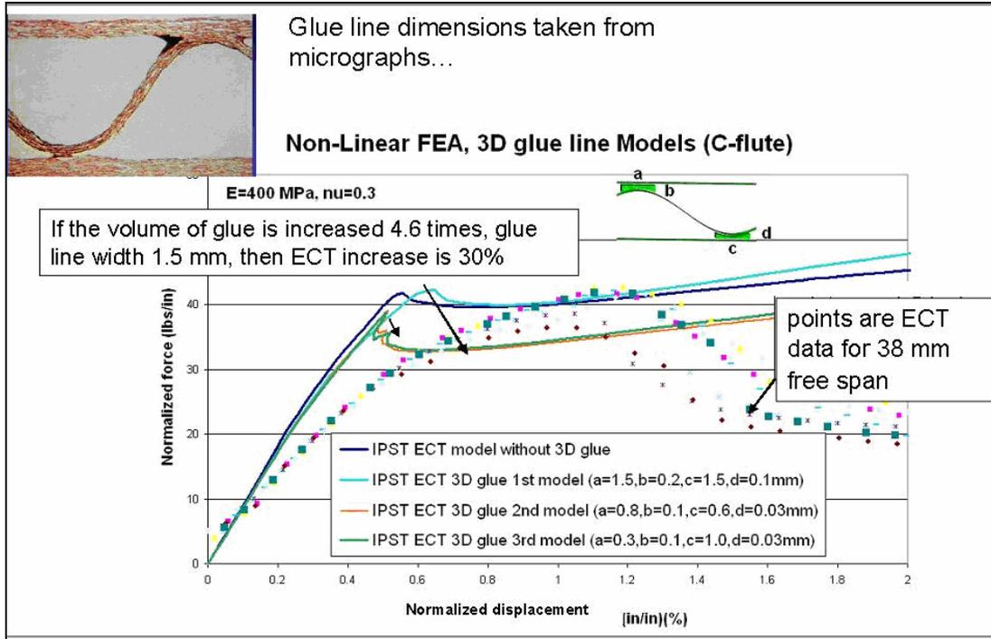
**Figure 2. Summary of FEA ECT results (specimen vertical free span 38 mm) with differing amounts of starch adhesive. Adhesive levels are indicated by widths a and c and thicknesses b and d. Micrograph insert taken from Skuratowicz, R., *Corrugating International*, 2003.**
