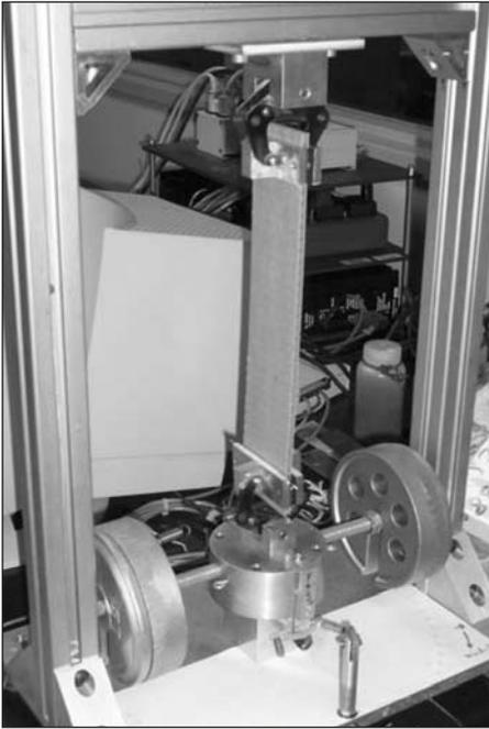
**Fig. 3** Photograph of the IPST torsion pendulum consisting of a freely rotating dumbbell fitted with a Hall effect sensor and clamps holding a twisting board test specimen.
