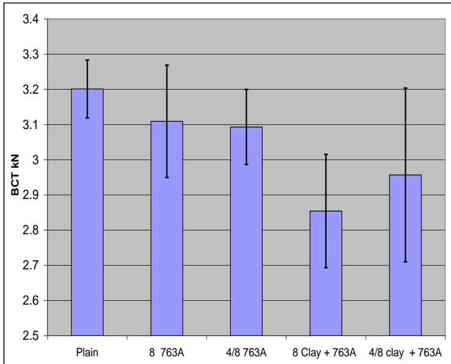
**Figure 6. BCT of the on-line coated linerboard test-box sample set.**
