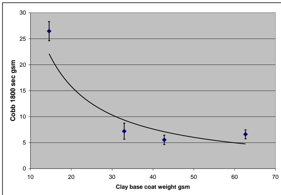
**Figure 2. Cobb 1800 s (30 min) water resistance as a function of the kaolin coat weight for laboratory coated linerboard. Error bars represent 95% confidence intervals.**
