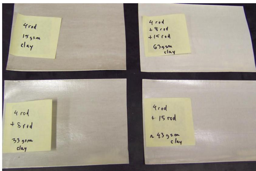
**Figure 1. Photographs of wire rod applied kaolin clay coatings on linerboard at various coat weights as indicated.**
