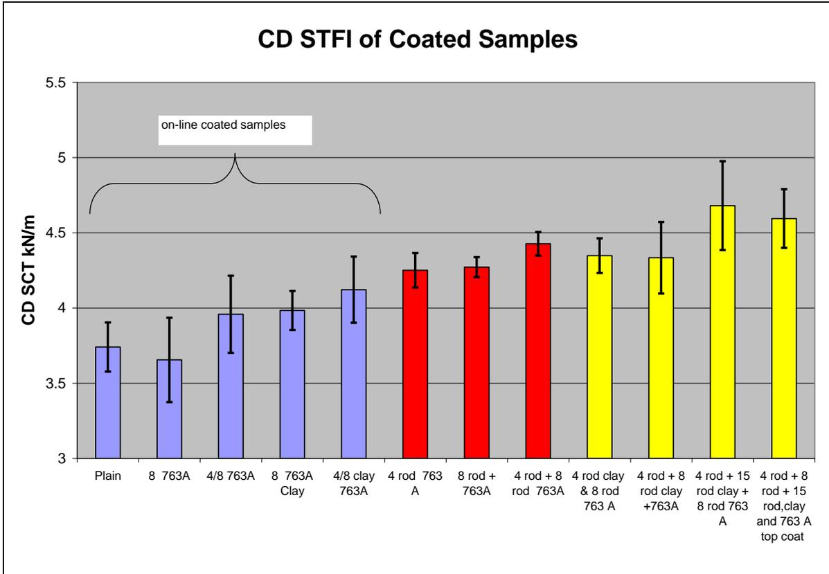
**Figure 3. Compression strength for linerboard samples, production and laboratory coated sample sets. Blue bar data are production coated, red bars laboratory drawdown coated with polymer only, yellow bars are laboratory coated with clay base and polymer top coat.**
