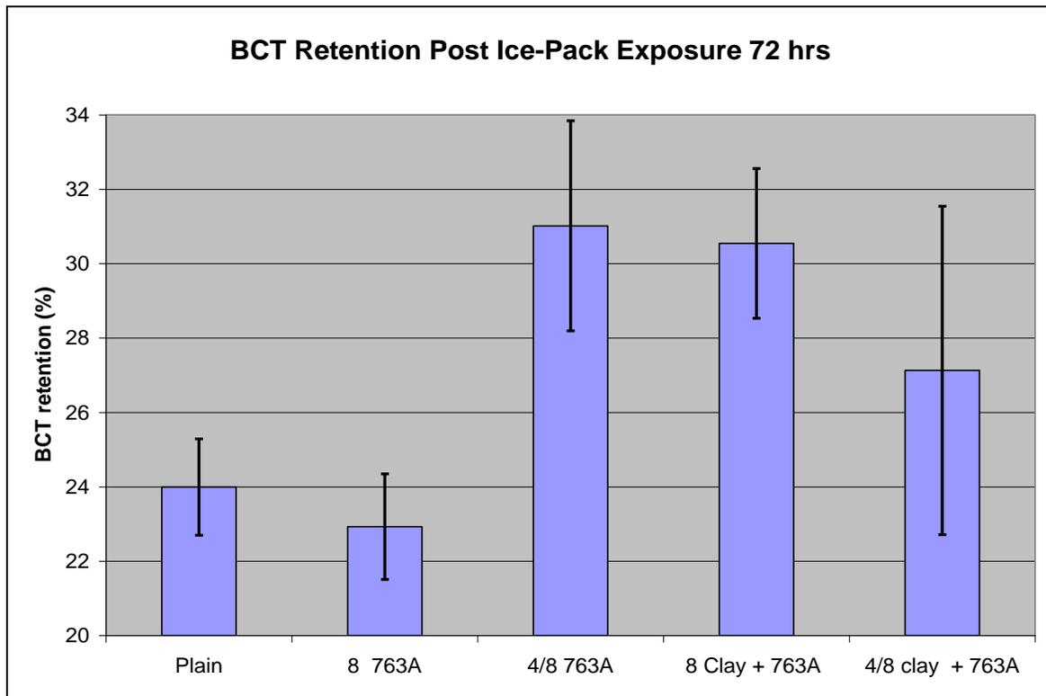
**Figure 9. BCT retention for the HSC coated linerboard box set after 72 hours of ice-pack exposure.**
