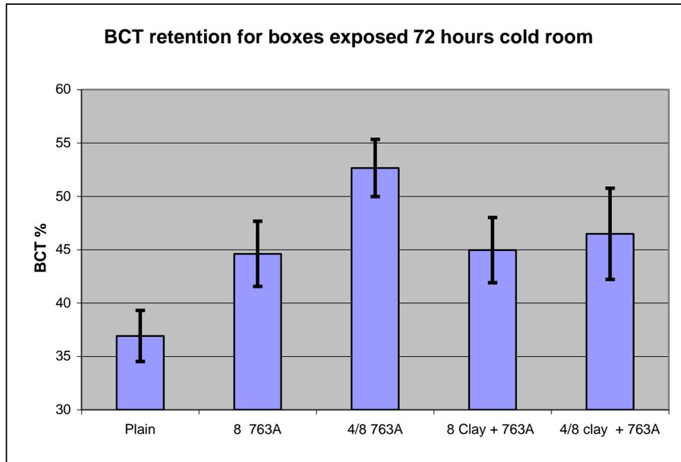
**Figure 7. BCT retention of the coated corrugated samples set after exposure to a high humidity cold room environment.**
