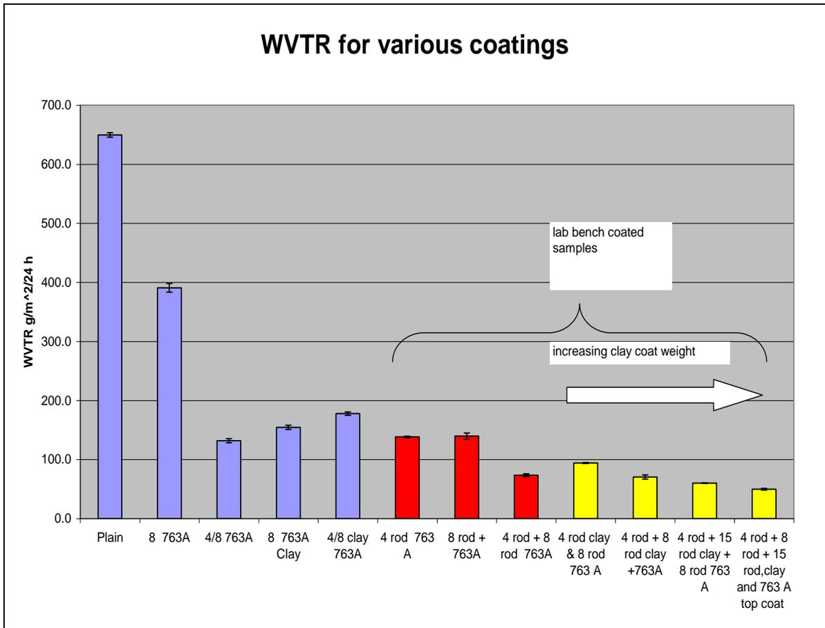
**Figure 4. WVTR for various coatings showing the effects of a clay base coat on 42 lb/msf linerboard. Color coding for data bars is the same as for Fig. 3.**
