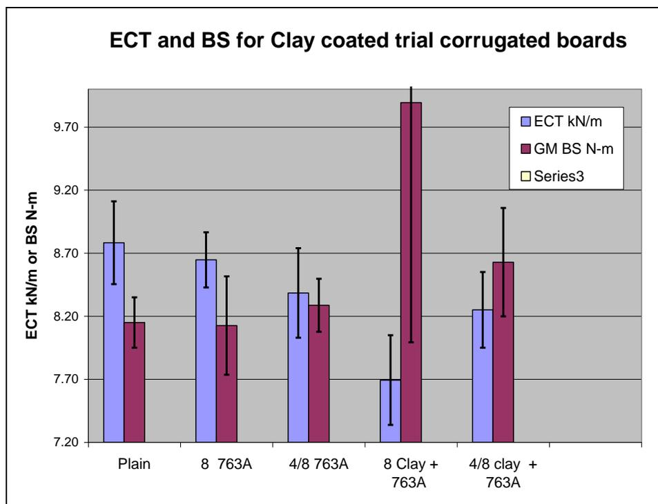
**Figure 5. Edge crush (ECT) and 4-point bending stiffness (BS) results for the corrugated board set.**
