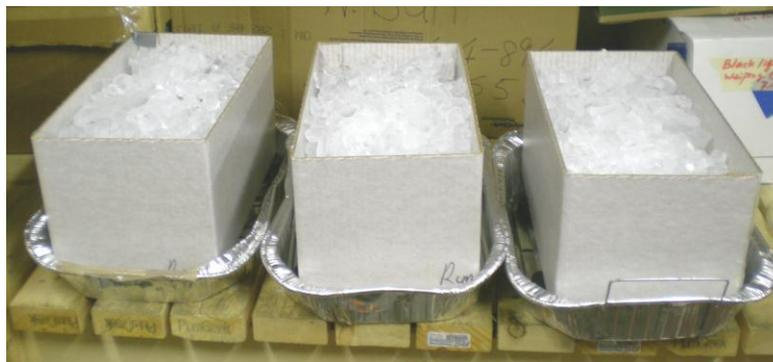
**Figure 8. A subset of the HSC coated linerboard boxes undergoing an ice-pack test in a cold-storage room.**
