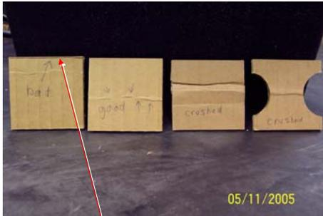
T 839 can have sample compressions along the edge, have to check samples after each test to ensure crease failure occurs between clamp faces
