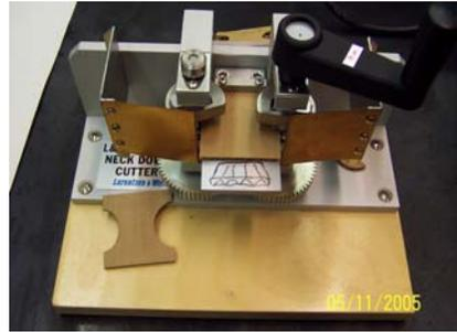
L&W neckdown ECT sample cutter, localizes compressive failure
