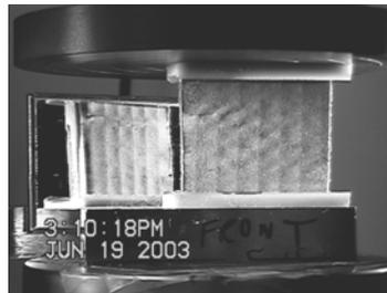
IPST investigations span length, loading rate and of liner inter-flute buckling – sample shot of AC board undergoing ECT
