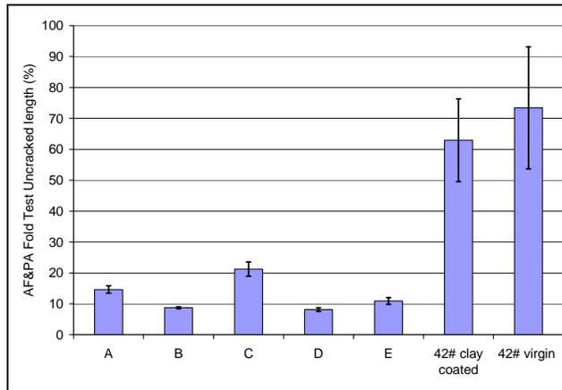
**Figure 6. Intact fold length (%) measured using the AF&PA nip technique.**
