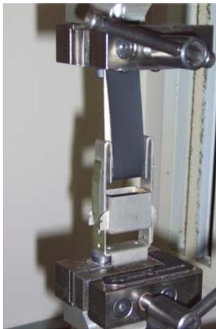
**Figure 4. Strip sample looped around the Finch cup dowel to measure the stretch to break with the sample in curved geometry.**
