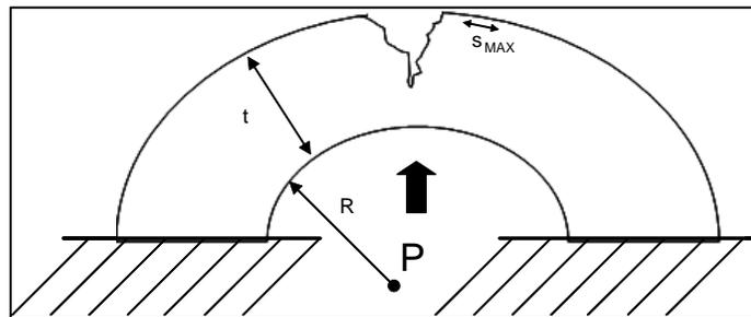
Figure 1. Schematic of fold cracking of a beam. Fissures start at the surface where strains are largest.
