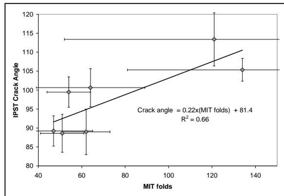
**Figure 8. IPST crack angle versus MIT folds for the sample set.**
