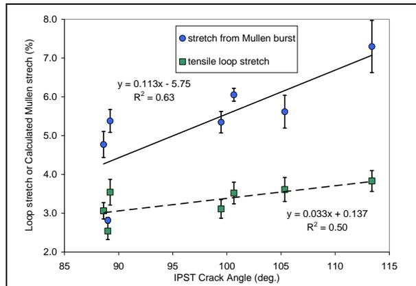
**Figure 10. Comparison of curved geometry stretch to break measurements with IPST Crack angle.**
