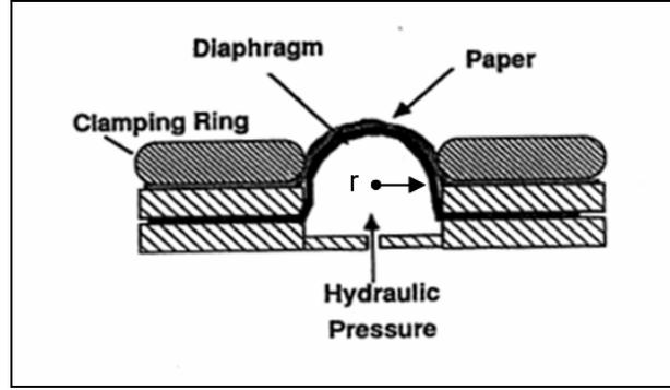
**Figure 5. Mullen burst test also has the test specimen subjected to high strain in curved geometry.**
