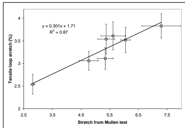
**Figure 9. Comparison of tensile loop stretch and stretch form Mullen and TSO measurements**
