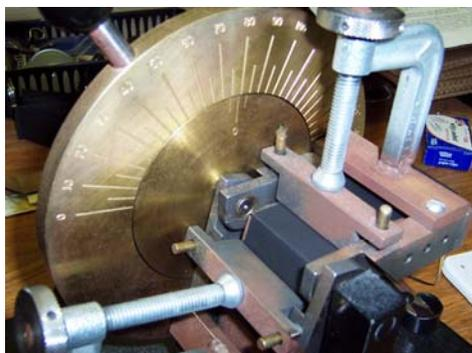
**Figure 2. Photograph of the IPST crack angle tester, the sample is progressively folded to larger angles until the fibers underneath show through the blackened top surface.**
