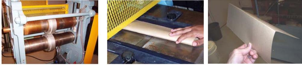
**Figure 3. Use of the AF&PA (Honshu) fold crack tester. Loosely folded over samples are sent through a pre-set nip of rotating anvils and the resulting sample is sighted along the fold to calculate the % length of cracked sample.**
