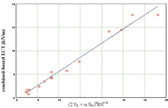
Figure 5) ECT vs STFI with Bending Stiffness
