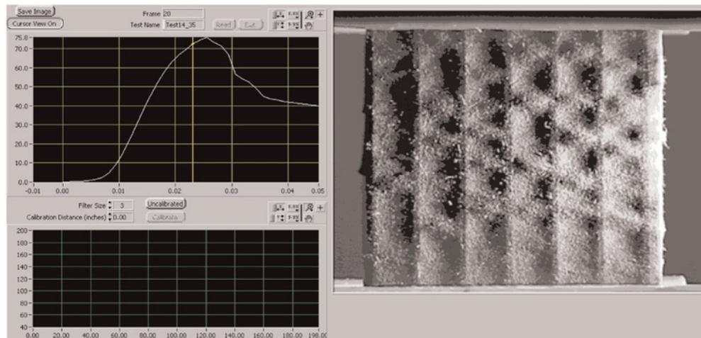
Figure 7) Considerable inter-flute buckling with 35-26-35 combined-board. Load displacement curve with the cursor corresponding to the photograph is shown on the left.
