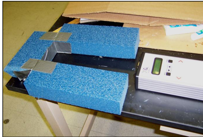
Figure 1. Improved foam sample support and BQM used in the measurements. Boards are placed with flutes perpendicular to the length of the BQM, the BQM is placed on top of the samples suspended by the foam blocks. Test boards are vibrated along their MD by the BQM, the frequency and amplitude of the test board's sympathetic vibration is converted to a shear stiffness numeric output.
