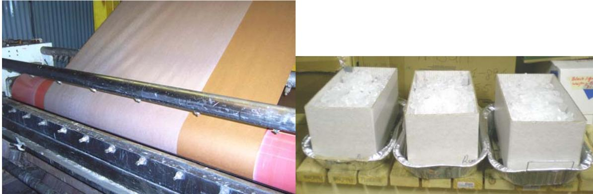
**Figure 3. Applying kaolin coating onto linerboard (left) followed by ice pack testing for BCT retention.**
