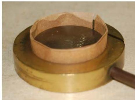
Ring Crush specimen after testing; buckling and rolling edges clearly visible
